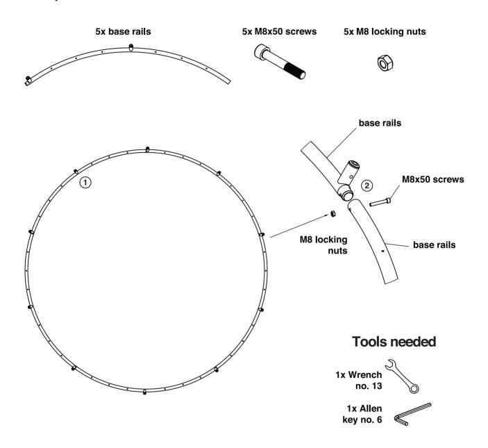
Place the base rails on the floor (1).
