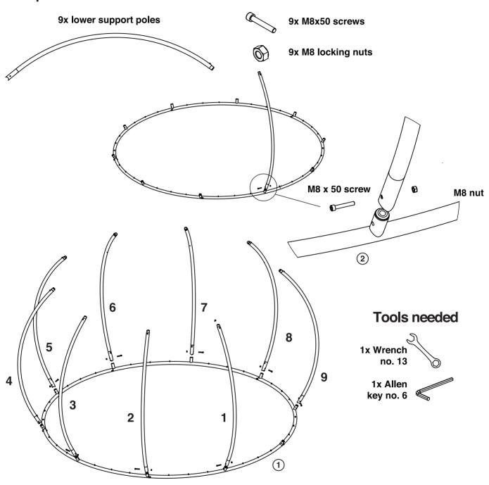
Mount the lower support poles (1). Identify the lower poles by the pre-mounted pin at one end and the circular milling at the other.
